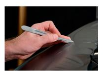
**Air bubbles:** Air and fluid bubbles should not be punctured. They disappear within a few days. Bubbles that are too large can be punctured with a very fine syringe needle.
