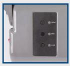
SELECT the heat temperature. Low- 110 degrees Medium- 120 degrees High- 130 degrees The temperature light will turn GREEN when proper temperature is reached.
